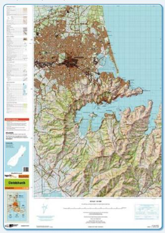
The Topo50 maps are easily distinguishable from the current NZMS260 series maps. They feature the green and orange branding, are printed in A1 portrait format and have new sheet numbering (see the example shown).
