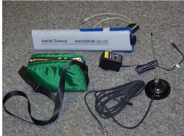
Wandatrak Kit shown above, the Regal 1000 receiver in the green pouch, charger plus both antennas, Directional Yagi in grey sleeve and vehicle mounted on cylindrical magnetic base.
