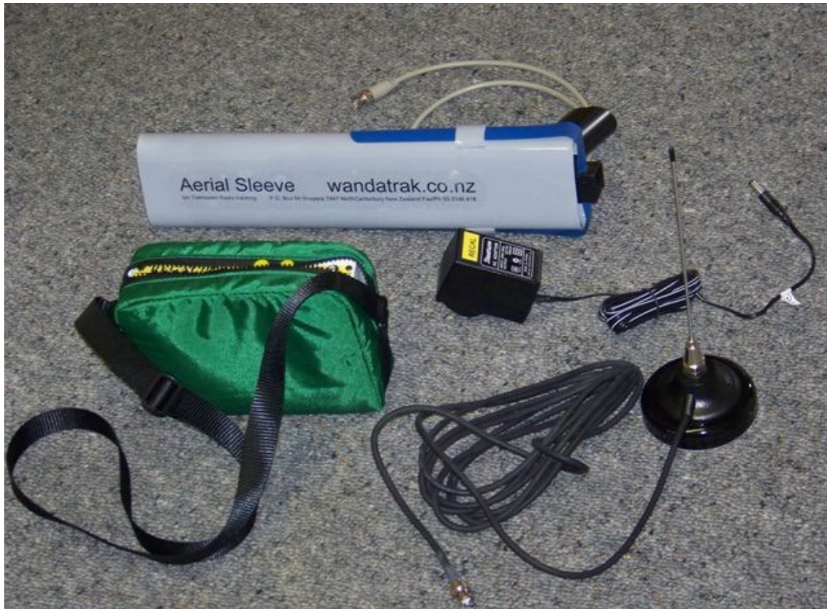
Wandatrak receiver kit shown above, the Regal 1000 receiver in the green pouch, charger plus both antennas (directional Yagi in grey sleeve and magnetic base whip antenna).
